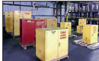
FLAMMABLE STORAGE CABINETS
